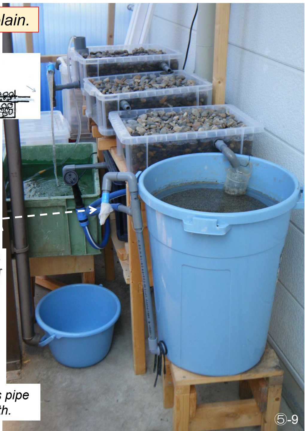
Up-flow roughing filter
